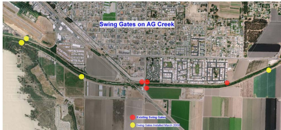
Figure 1. Swing gates to control vehicle access on levee: red dots indicate gates already installed, yellow dots to be installed shortly.
