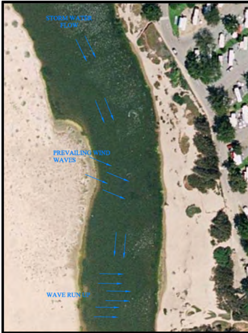
Figure 3. Illustration of Causes of Erosion
